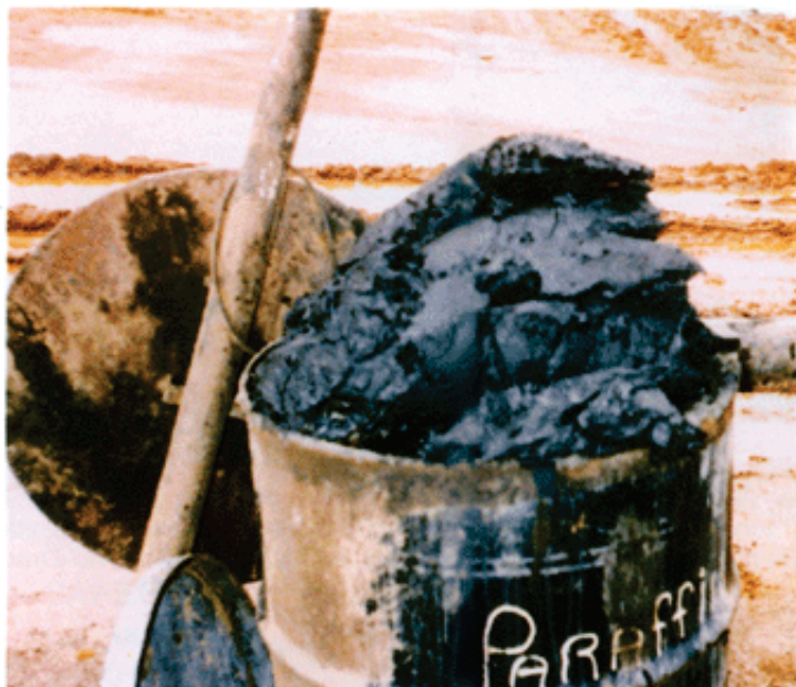
Operator was pigging a 4" 4-mile pipeline three times per week, getting a bbl to a bbl 1/2 of hard paraffin, which had to be disposed.
